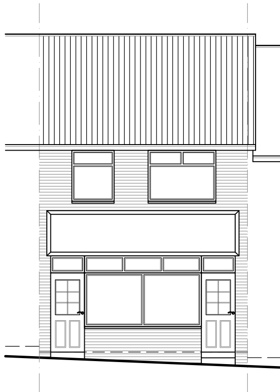
EXISTING ELEVATION (From Windsor Rd) Scale 1:100
